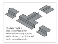
channel) it can interface with the levels at which contaminated land cavity barriers are commonly installed in the external walls. Water can safely discharge and gas tight integrity be maintained.
