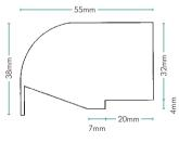
Over Fascia Ventilator OFV10, for roofs requiring the equivalent of a 10mm continuous gap. Suitable for roof pitches of 15 degrees upwards.
