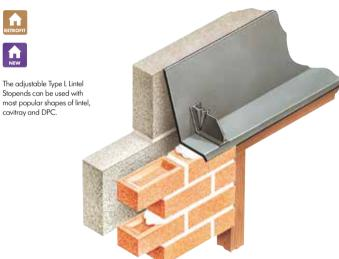
Stopends for application onto lintels, DPCs and Cavitrays to prevent water discharging off ends into cavity.
