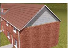
Leeward suction can cause failure across the gable at its weakest point where the outer leaf is sitting on a conventional DPC
