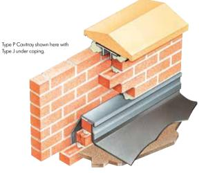
To provide protection against damp penetration where a parapet wall rises above roof level.
