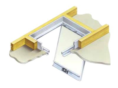
To provide access with a fire integrity rating of two hours into a roof space.
